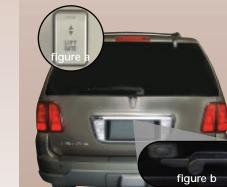
To open the optional power liftgate, either push the overhead console button (figure a), pull the outside release handle (figure b), or press the LIFT GATE button on your key fob.
